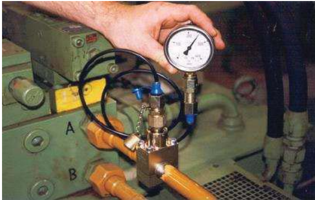
Installation on pressurized pipe serv-Clip® 1
