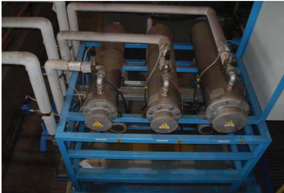
Picture 1: Pressure measurement at a flow pickling line for grease oils with serv-Clip ® -1 and pressure sensor DS-1-A-400-1/4" fluid-Check ®
